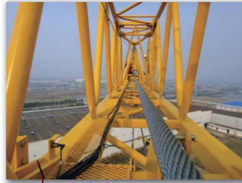
Catwalk and independent safety rope along the full 75m jib give the highest safety to walk along the jib
