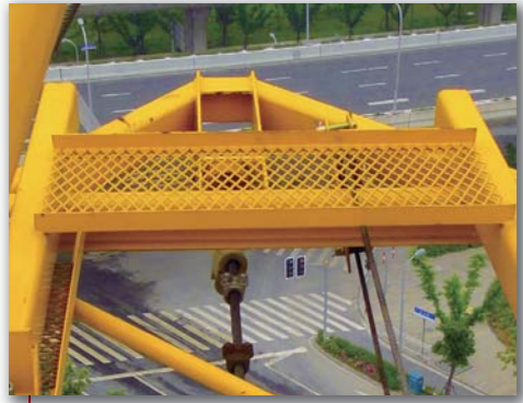
Platform for operations at the jib nose
